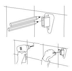
1. Mark, drill, plug and screw the wall brackets in the required position.
