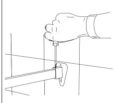
Lock the grub screws when the track is fully assembled in position.
