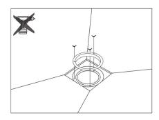
(4) Reassemble the 3 screws of the steel ring to the waste trap always using standrad screwdriver.
